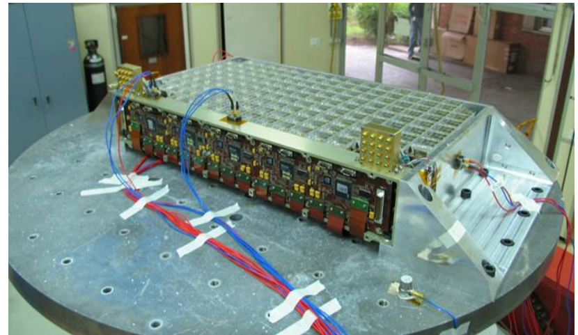
setup for grid vibration test
