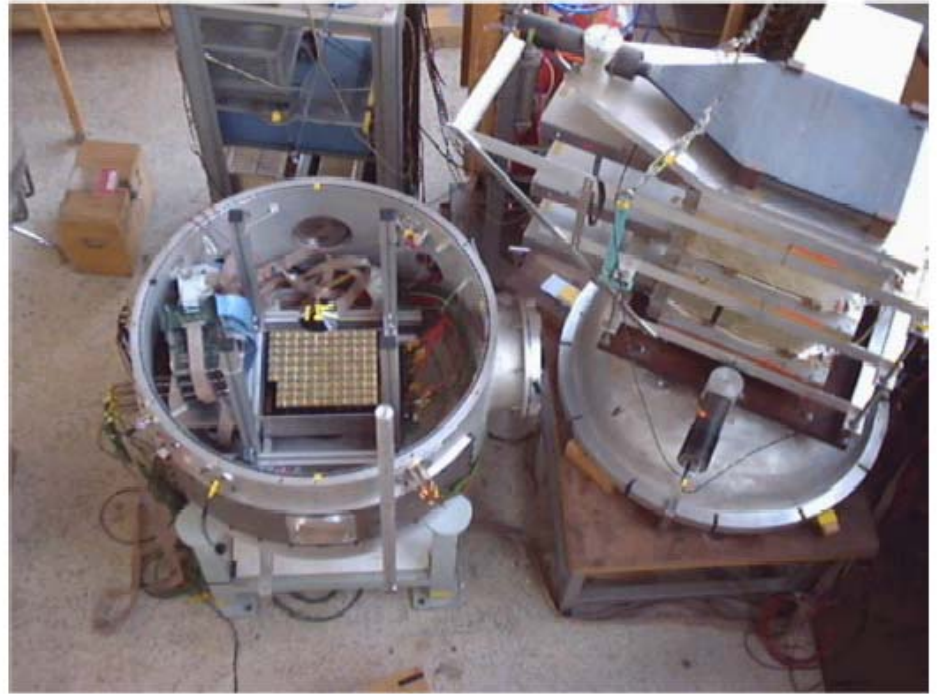
RICH prototype at cosmic-ray testing in Grenoble
