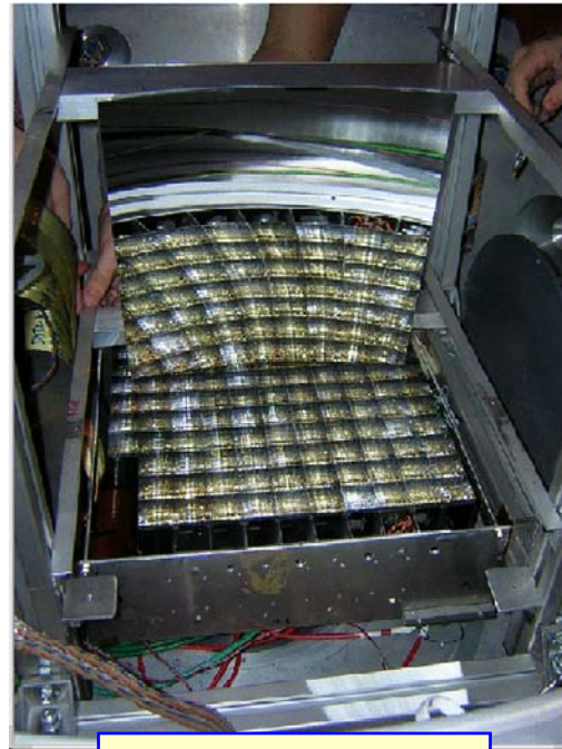
RICH prototype with mirror segment
