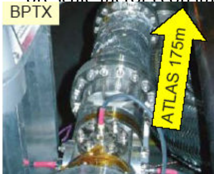
Beam Pickup: at \pm 175\text{m} from ATLAS Trigger on filled bunch Provide the reference timing
