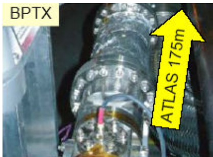
Beam Pickup: at \pm 175\text{m} from ATLAS Trigger on filled bunch Provide the reference timing
