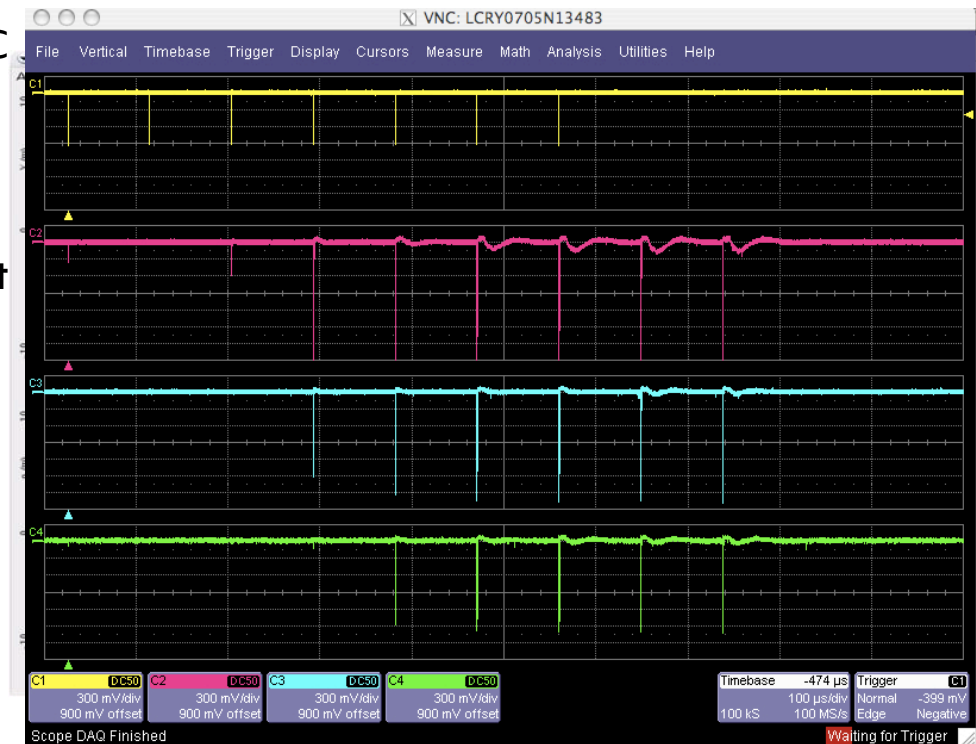
Oscilloscope traces from beam pickup (yellow) and min.bias scintillators for single injected bunch
